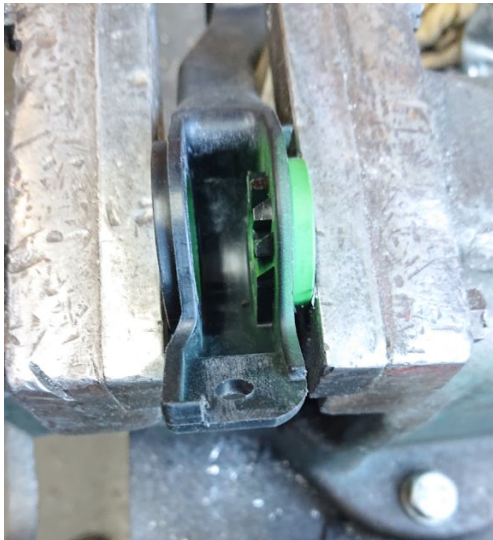
Figure 3: Pedal arm drilling
