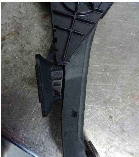
Figure 6: Pedal Stop ground back to provide additional travel
