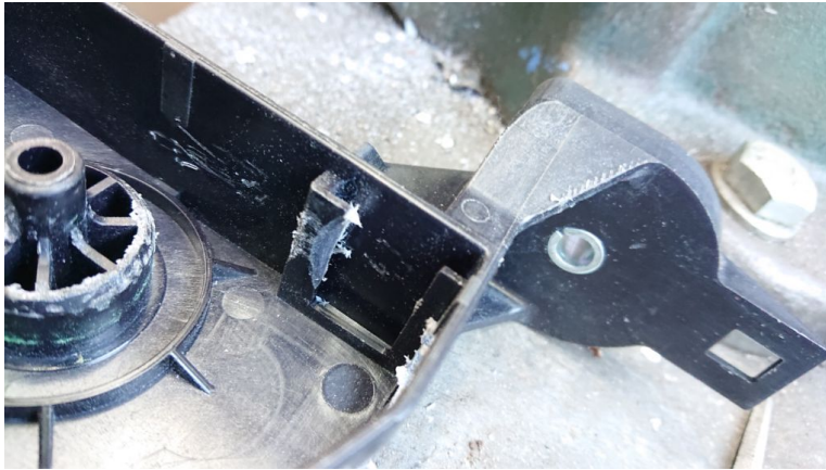
Figure 5: Relieving the plastic casting for the M5 bolt head
