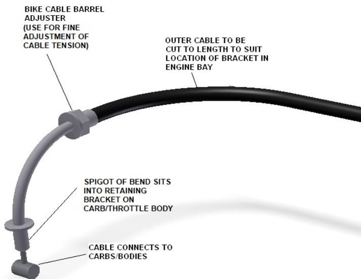
**Figure 1:** Typical arrangement using the 90deg bend provided in the kit to nicely guide the cable away from the carbs horizontally. The lower part of the bend sits into the 'C' shaped throttle bracket on most typical bike carbs and throttle bodies. The 6mm diameter nipple on the end of the inner cable can either be a fixed nipple (using our pre-made inner cable as supplied in the full cable kit) or the supplied solderless nipple. Inner and outer cable lengths will need to be trimmed to suit.
