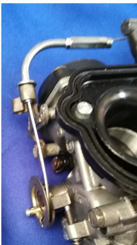
**Figure 2 (left):** Cable routing for a bike carb application - applies to throttle bodies also. Note that whilst the photographed carbs (ZX6R) have the linkage on one end, the cable arrangement would be the same for carbs with the linkage inbetween carbs.
