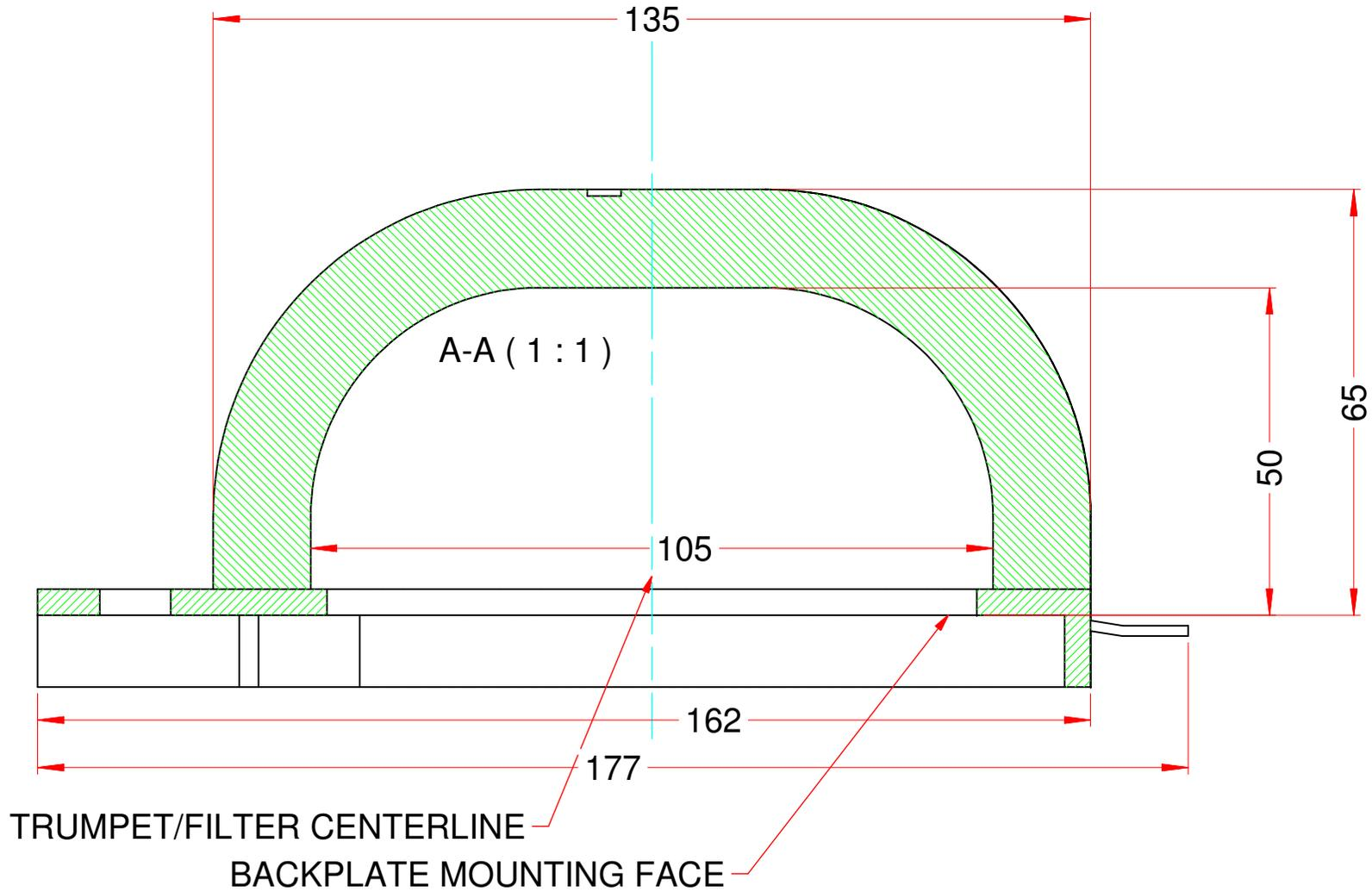
NOTE! CONSTRUCTION OF THE FILTER ELEMENT, WIRE MESH SUPPORT AND AS SUCH SOME DIMENSIONS MAY HAVE SLIGHT VARIATIONS
