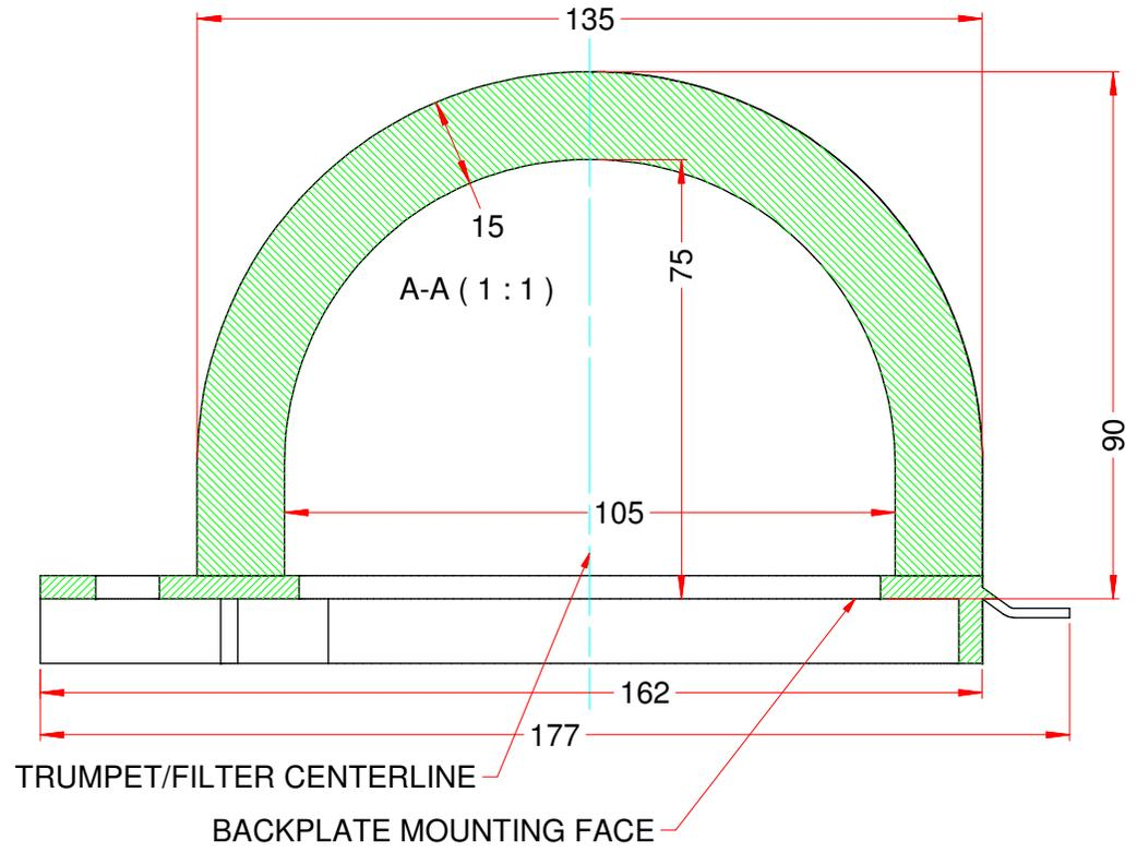
NOTE! CONSTRUCTION OF THE FILTER ELEMENT IS FOAM WITH WIRE MESH SUPPORT AND AS SUCH SOME DIMENSIONS MAY HAVE SLIGHT VARIATIONS
